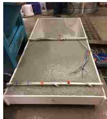
Figure 6-6 Preparation and casting process of UHPC overlay
