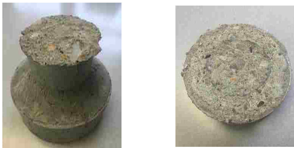
Figure 6-16 Test set-up and fracture mode for UHPC debonding test
