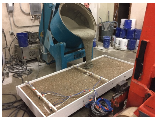
Figure 6-6 Preparation and casting process of UHPC overlay
