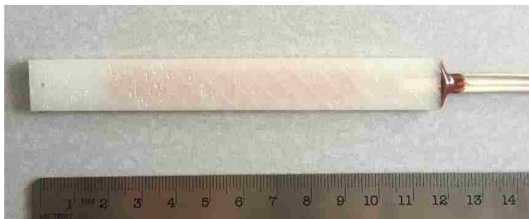
Figure 6-3 Embedded strain gauge for monitoring shrinkage deformation
