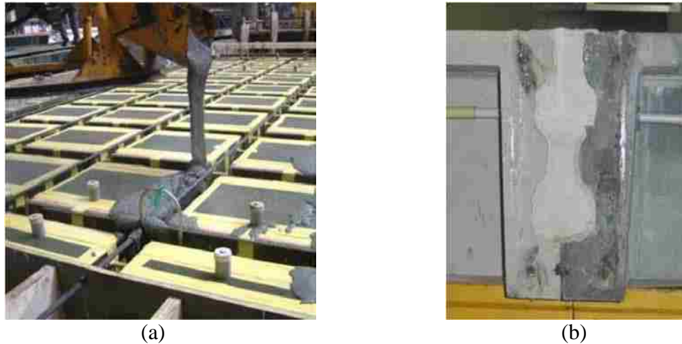
Figure 2-11 Model ribbed slab for validation tests. a) Casting - b) Cold joint (Toutlemonde et al., 2007)
